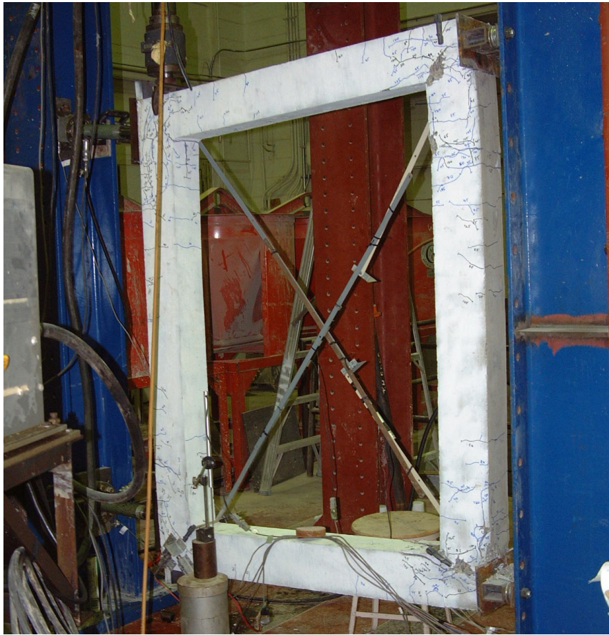
Fig. 7. Cracks observed in the moment frame at failure.
